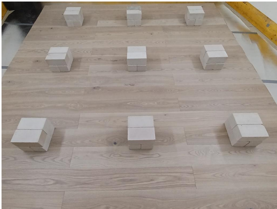
Figure 4: completed floor with weight load (situation during test)
