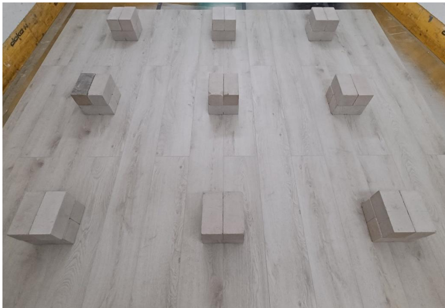
Figure 4: completed floor with weight load (situation during test)
